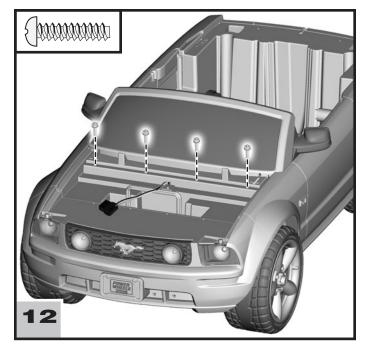
• Insert four #8 x  $^{3}/_{4}$ " screws into the dash assembly and tighten.
